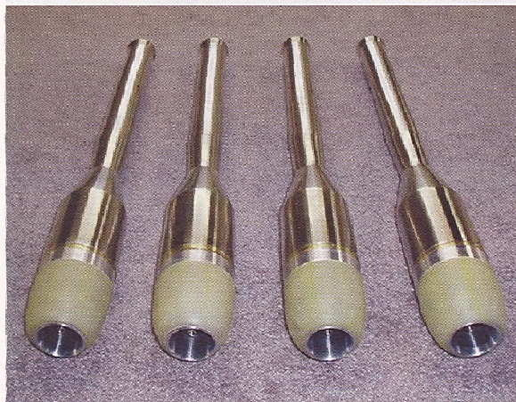
Completed pulse-jet engines attached to Bailey stainless-steel pipes.
